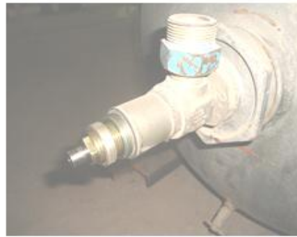
Fig 10 The pressure regulator
